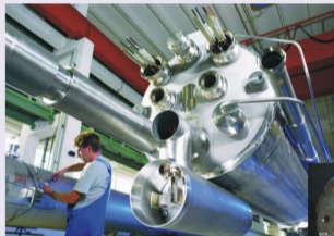
Scope: 416 Superconductive Dipole Magnets
